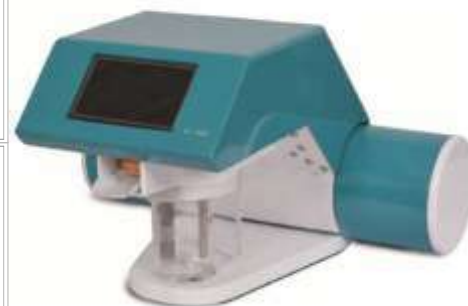
DAMAGED STARCH DEVICE
